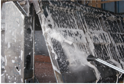
Wash and Degrease
